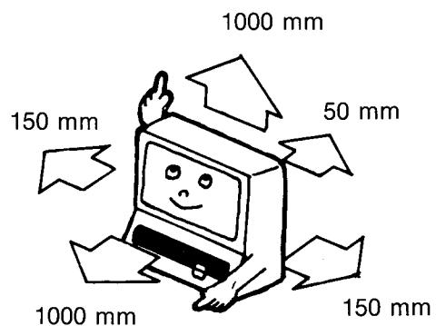
Do not allow curtains or other flammable materials to come into contact with the heater.
